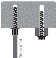
With the correct diameter drill bit, drill a hole to the correct depth (add at least one anchor diameter to the depth to prevent the fastener from bottoming out).
